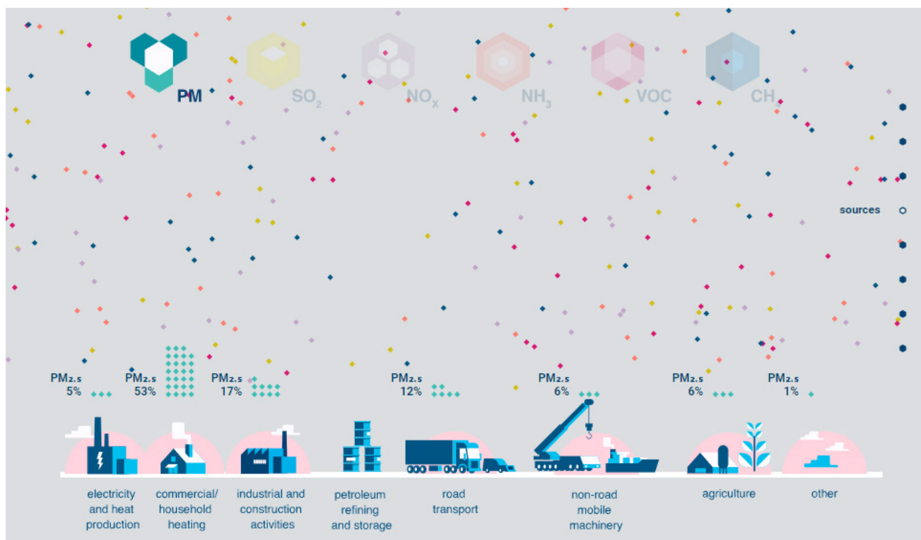
Figure 2. Sectoral contributions to PM 2.5 (Source: European Union emission inventory report 1990–2013, European Environment Agency)
